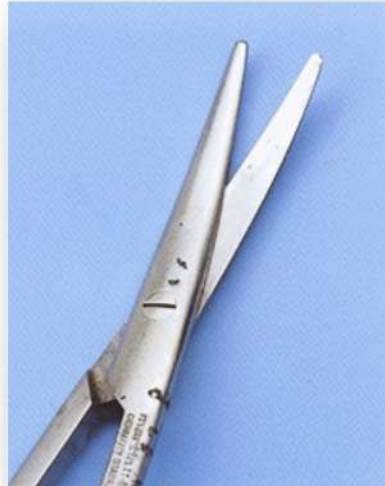
Figure 7: Chloride Induced Pitting
