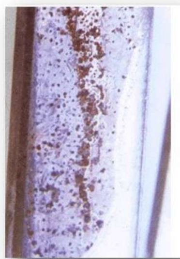
Figure 17: Pitting due to Caustic Solution—magnified
