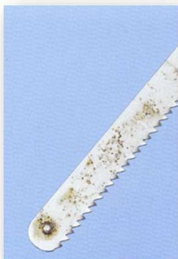
Figure 15: Discolouration and Rusting due to poor cleaning
