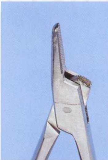
Figure 9: Stress Corrosion Cracking
