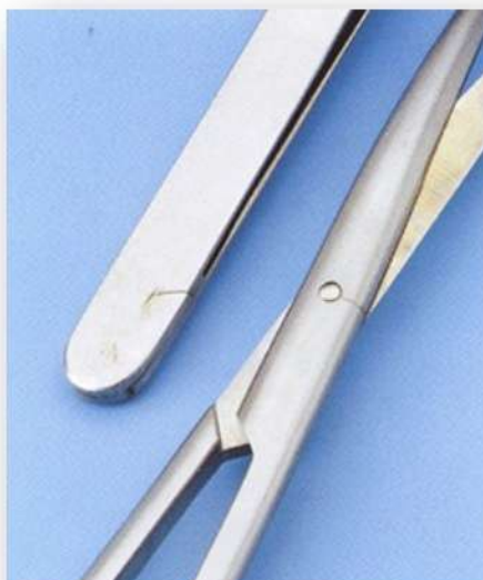
Figure 10: Stress Corrosion Cracking
