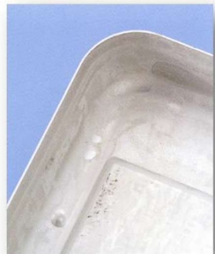
Figure 2: Corrosion of Anodised Aluminium
